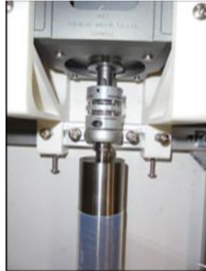
(b) Connection between motor, gear and the drum
