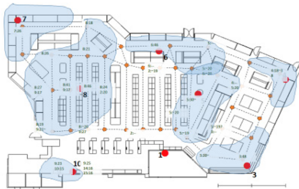
Figure 4 Communication Range of the Antennas
